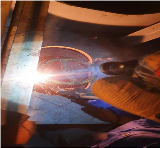
Having checked the situation, we found that the grease residues has hardened and we carry out heating on the cargo hold flap spindle and found to be succesful
