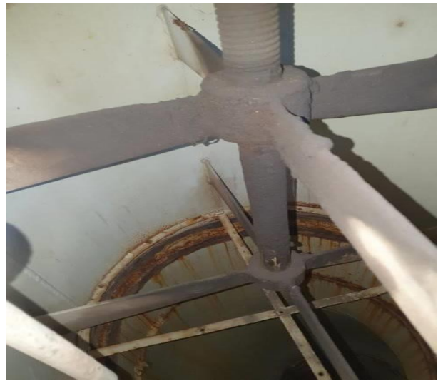
Having checked the situation, we found that the grease residues has hardened and we carry out heating on the cargo hold flap spindle and found to be succesful
